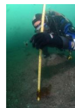
Figure 5 measuring the scour
