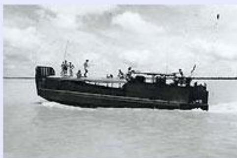
Landing Craft Mechanised 35-115 tonnes, versatile landing craft capable of carrying tanks and soldiers.
