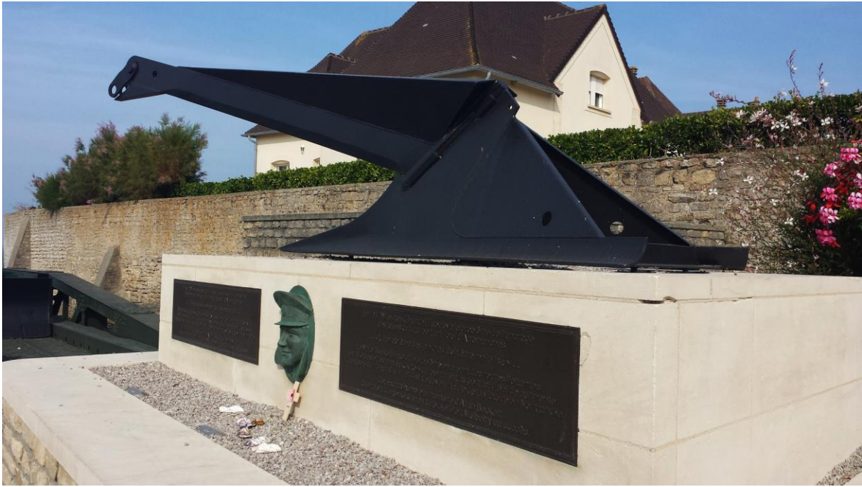
Figure 61 A replica Kite anchor used to provide a secure grounding for the bridge sections. (Martin Davies)
