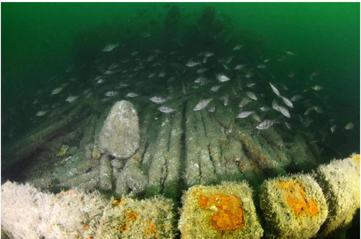
Figure 50 The square design of boilers is typical of a Liberty Ship (Martin Davies)
