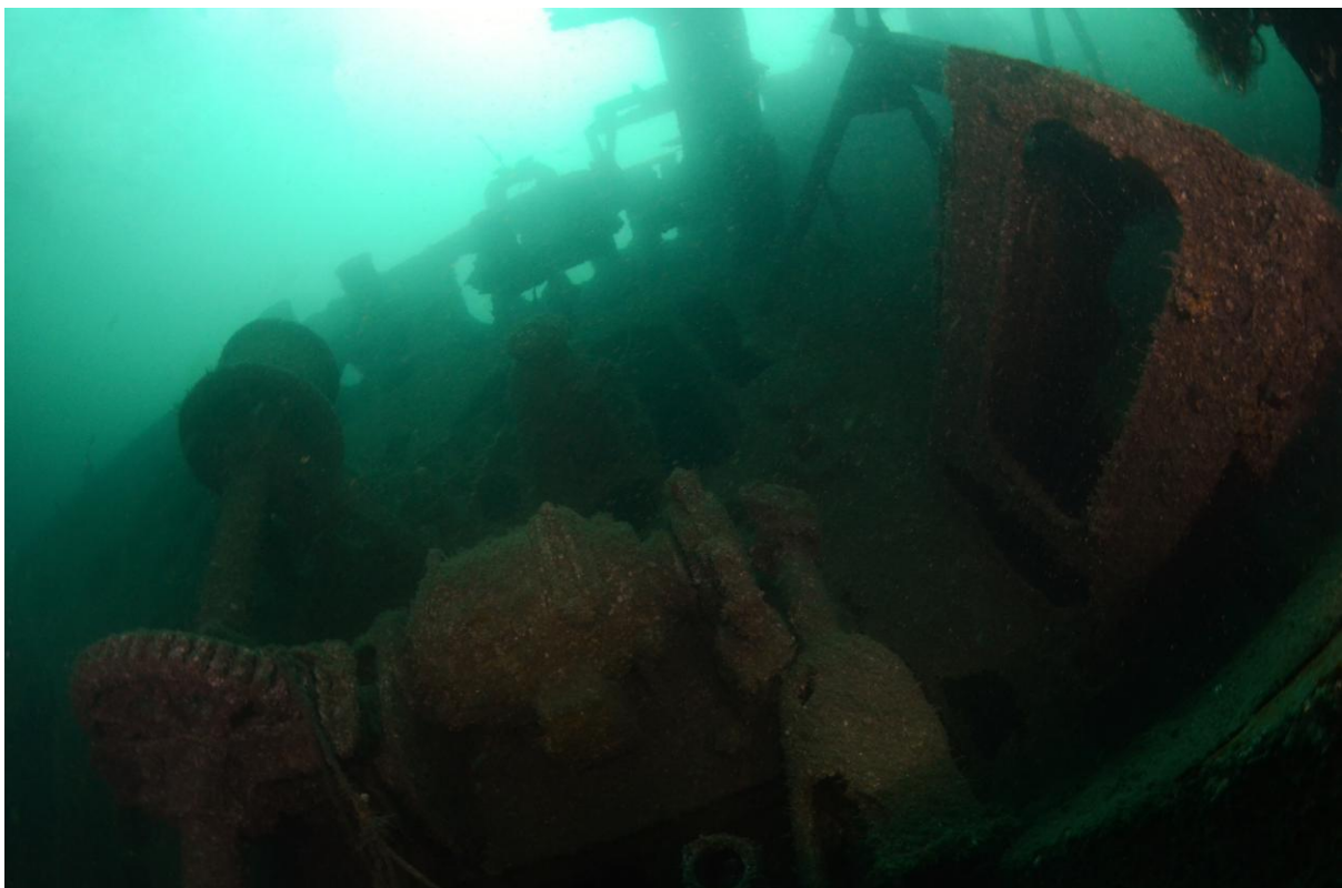
Figure 42 Looking up across the stern section the deck winches are remarkably intact. (Martin Davies)
