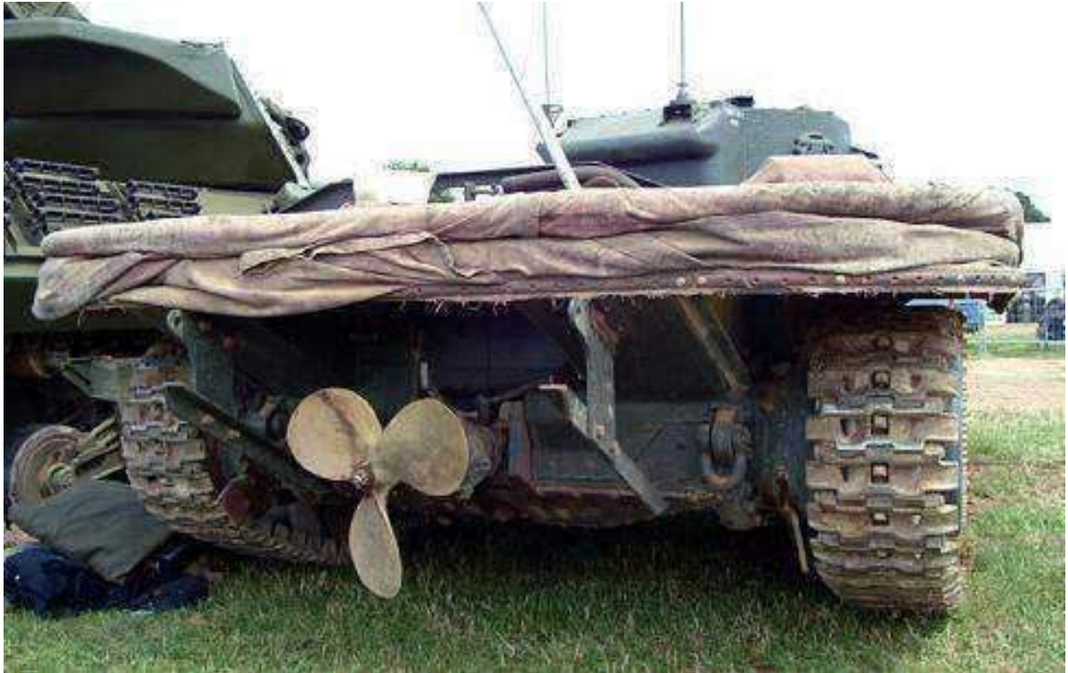
Figure 76 - Restored Valentine DD tank with propeller and canvas skirt.
