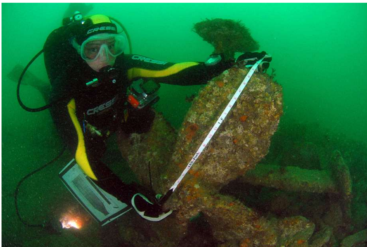
Figure 7 - Measuring the LCT propeller (Image Martin Davies)
