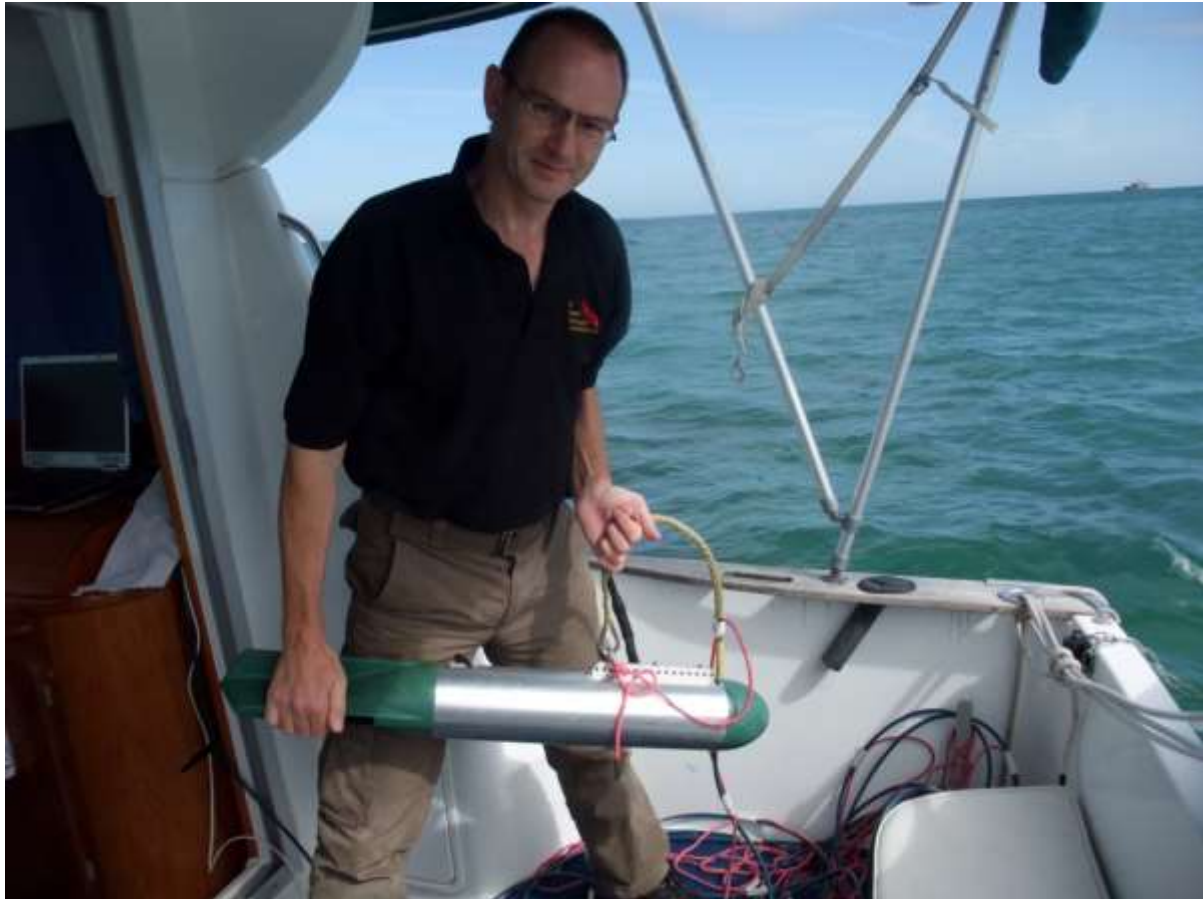
Figure 10 Diving Officer Martin Davies launching the side-scan sonar 'fish' (Image Alison Mayor)
