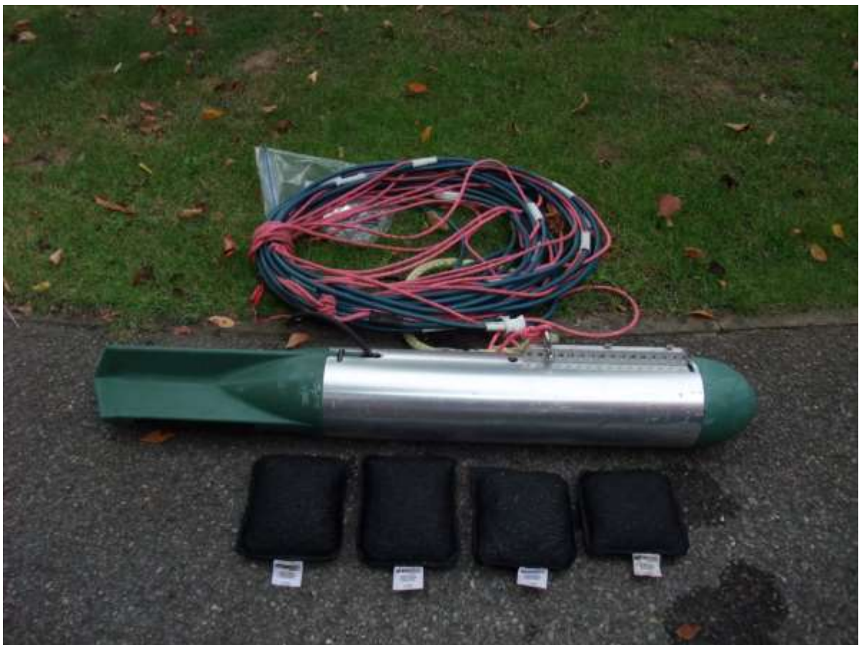
Figure 9 -Side Scan Sonar equipment kindly loaned by Nautical Archaeology Society (NAS)
