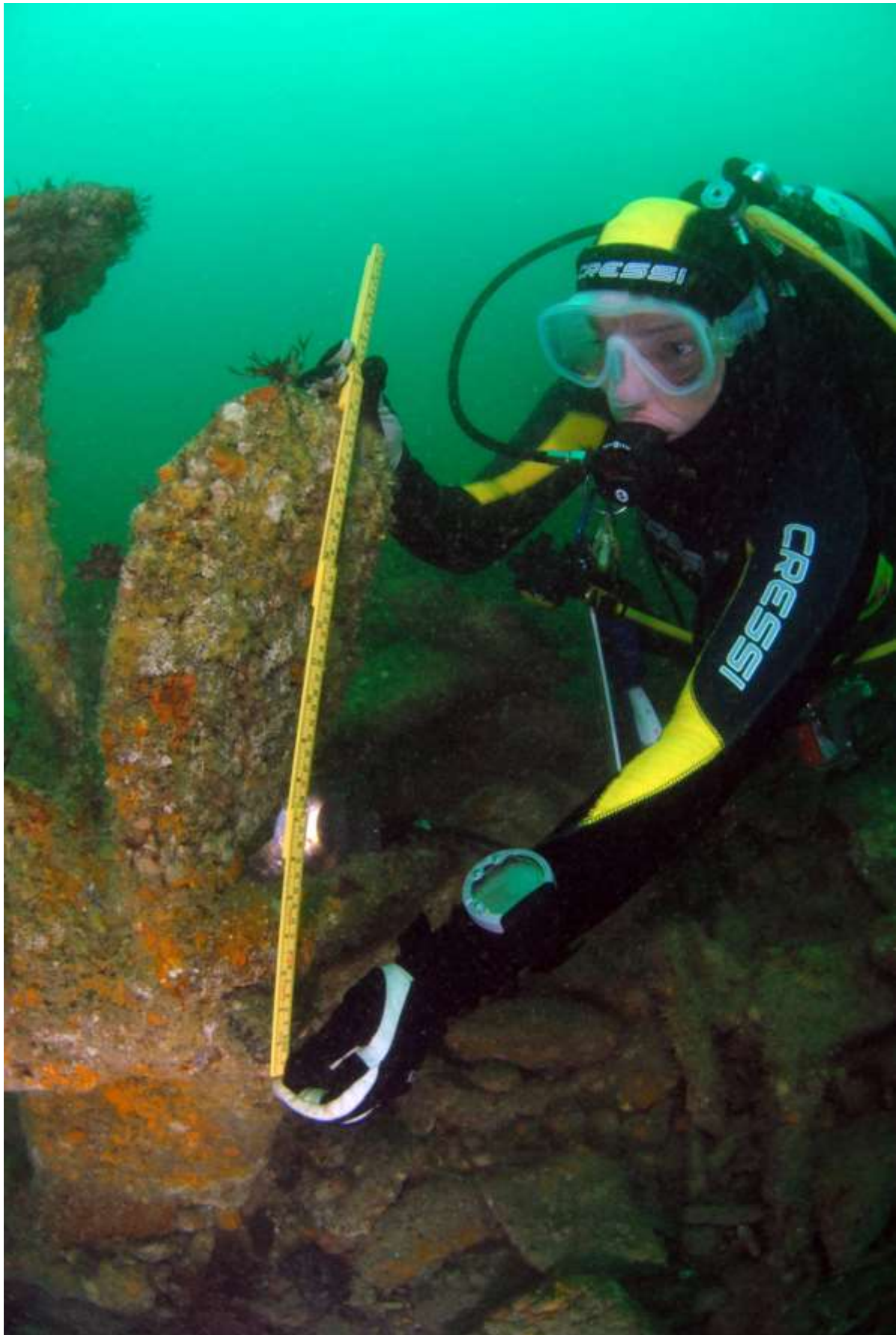
Figure 19 - Propeller - 4 blade and 37 inch diameter (Image Martin Davies)
