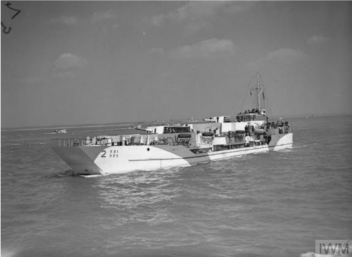
Figure 19. LCG 939 afloat (note the LCT flat bow of earlier Mk 4 hull conversions) (© IWM A 23754)
