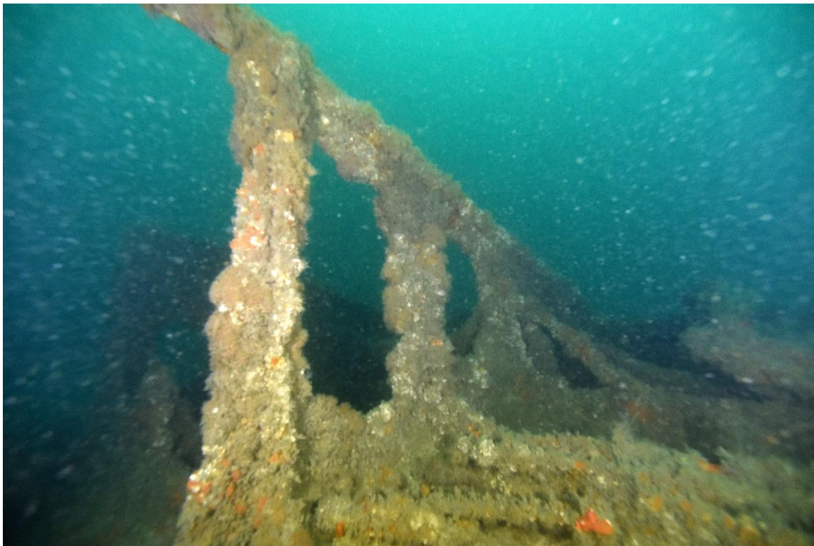
Figure 56. The upturned stern and one of the skegs of the vessel. (©Martin Davies)
