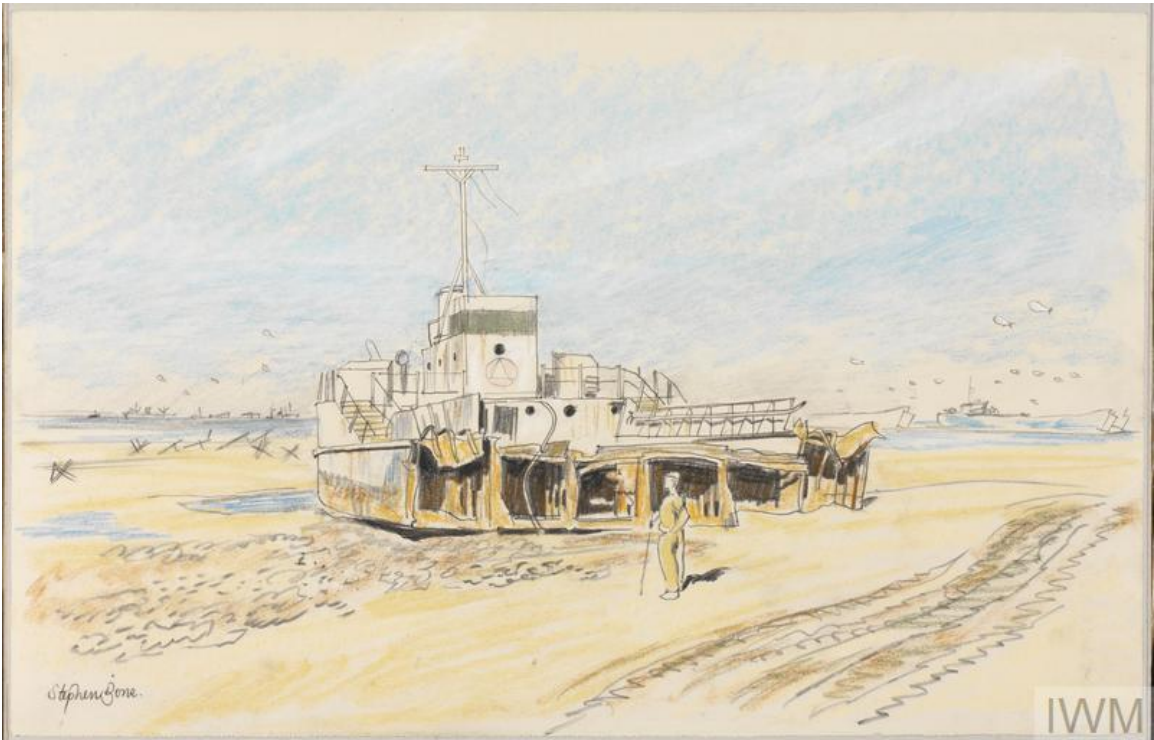
Figure 61. In this painted sketch the stern of a LCT lies rusting on the sand at low tide at Courseulles clearly showing the construction of the LCT Mk 4 hull. © IWM (IWM ART LD 4363)
