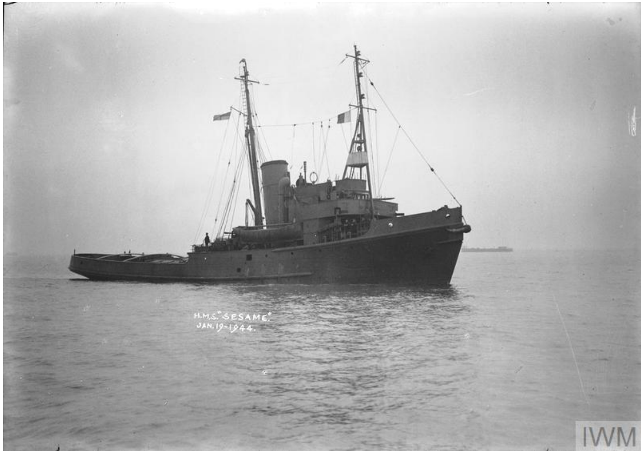
Figure 21 Photograph of HMRT SESAME January 1944. Note the stepped hull shape. (© IWM (FL 18913))
