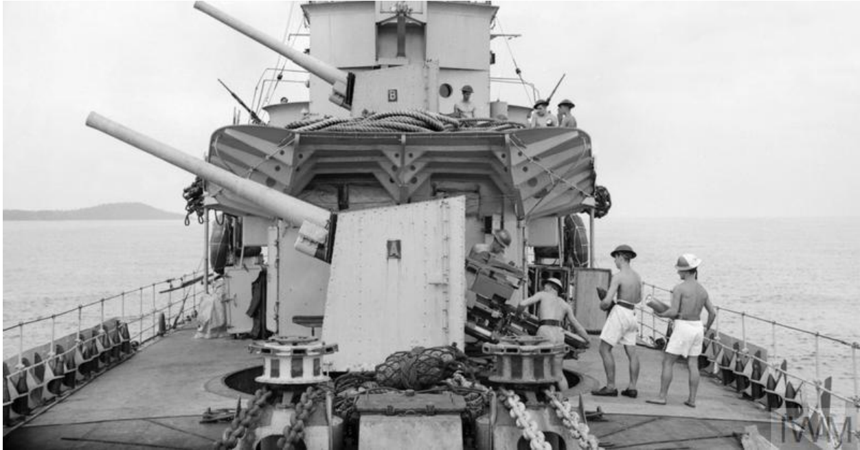
Figure 65 the forward 4.7-inch guns of HMS FOXHOUND, off Freetown, Sierra Leone, August 1943. (© IWM (A18772))
