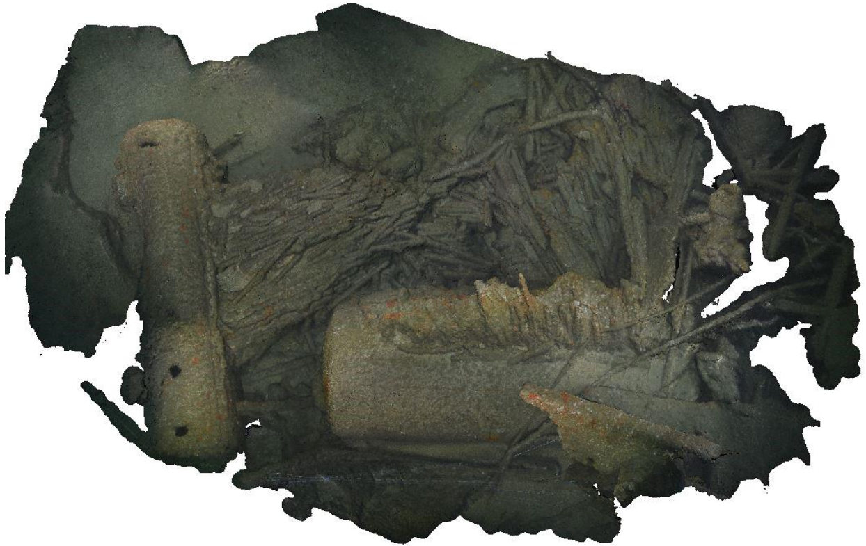
Figure 50 EA3234 Photogrammetry image of boiler debris - larger cylinder (steam drum) and smaller cylinder (water drum). (© Martin Davies)
