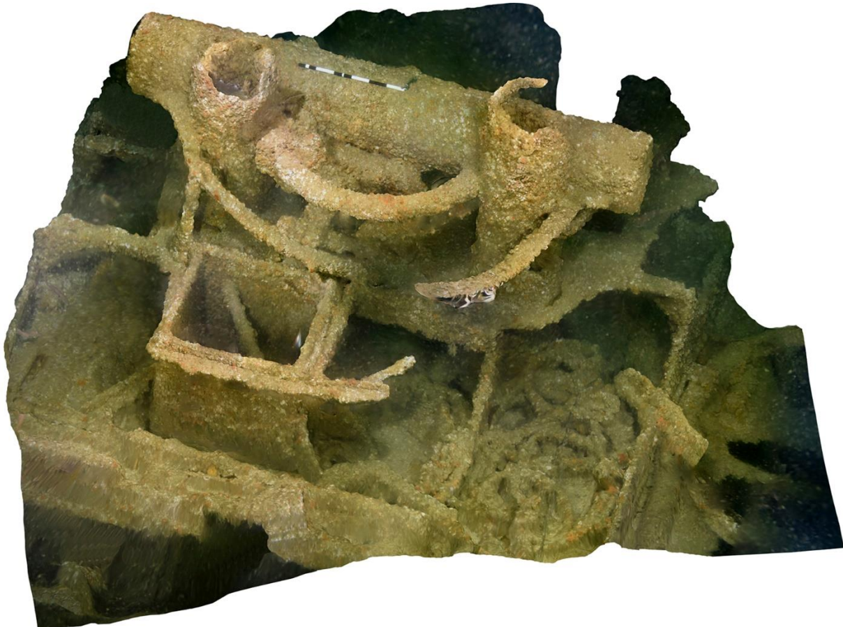
Figure 23 EA4360 Image from photogrammetry model. Towing stanchion from port looking forward. (© Martin Davies)
