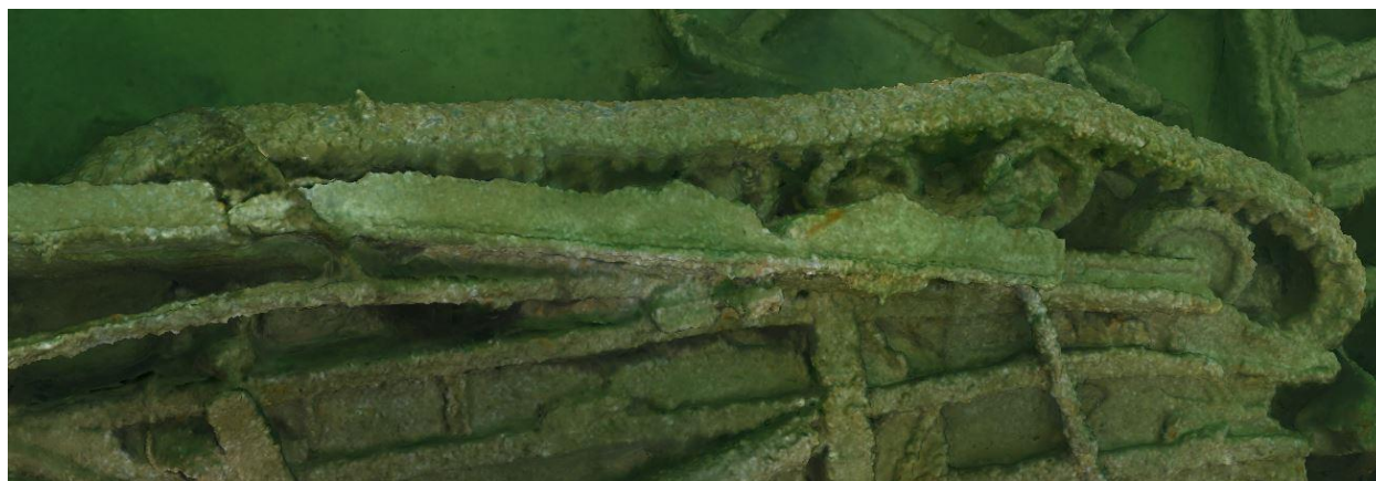
Figure 36 Tracks and wheel and suspension assembly of upside-down Sherman tank. (© Martin Davies)
