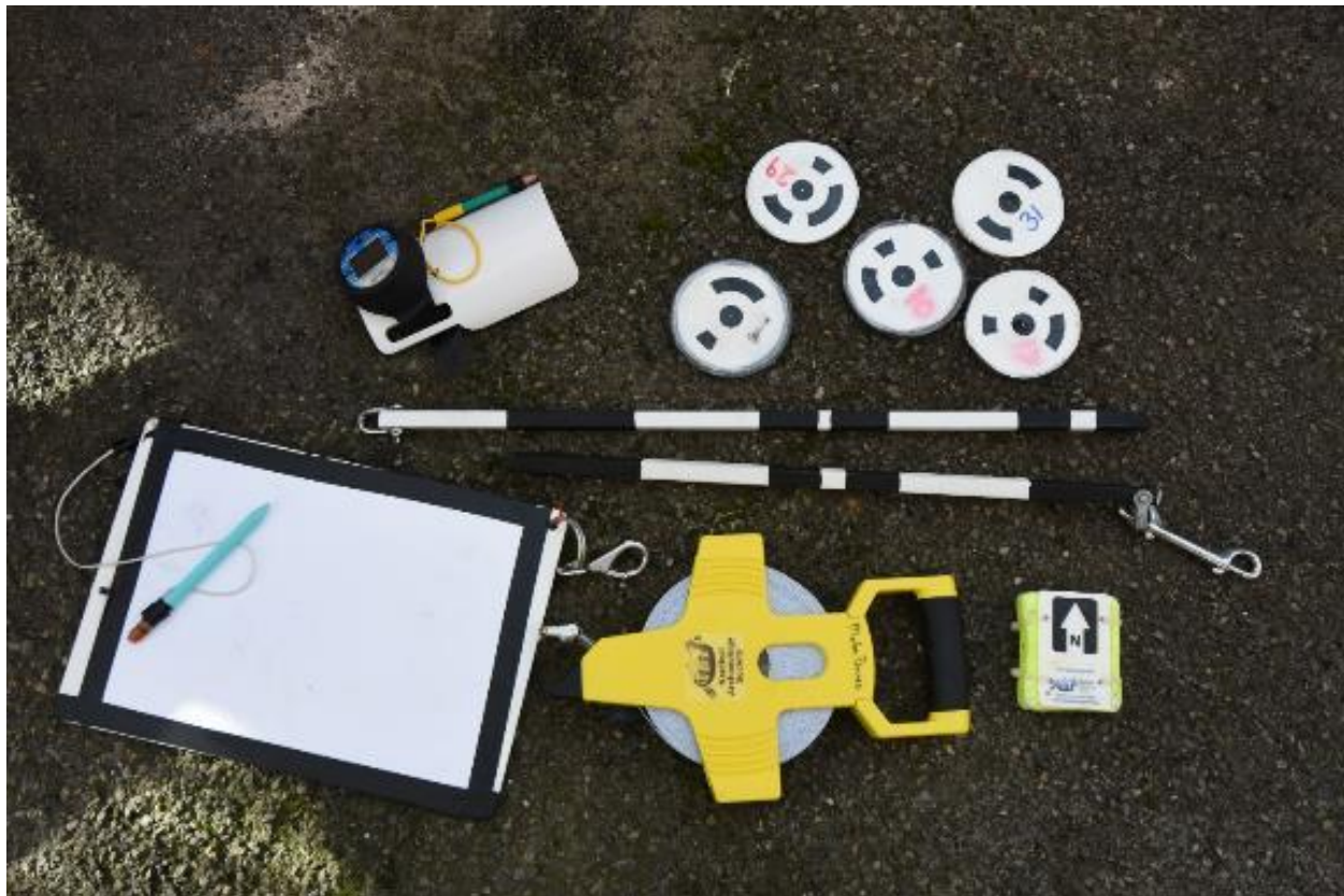
Figure 11. Typical survey equipment used for the project. (© Martin Davies)
