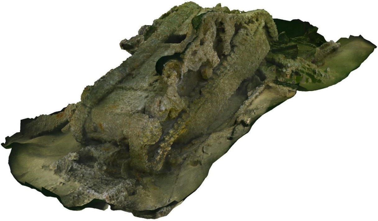
Figure 38 Front and right-hand side view of a Stuart M5A1 tank. Note the raised engine section which distinguishes it from a Stuart M3. (© Martin Davies)
