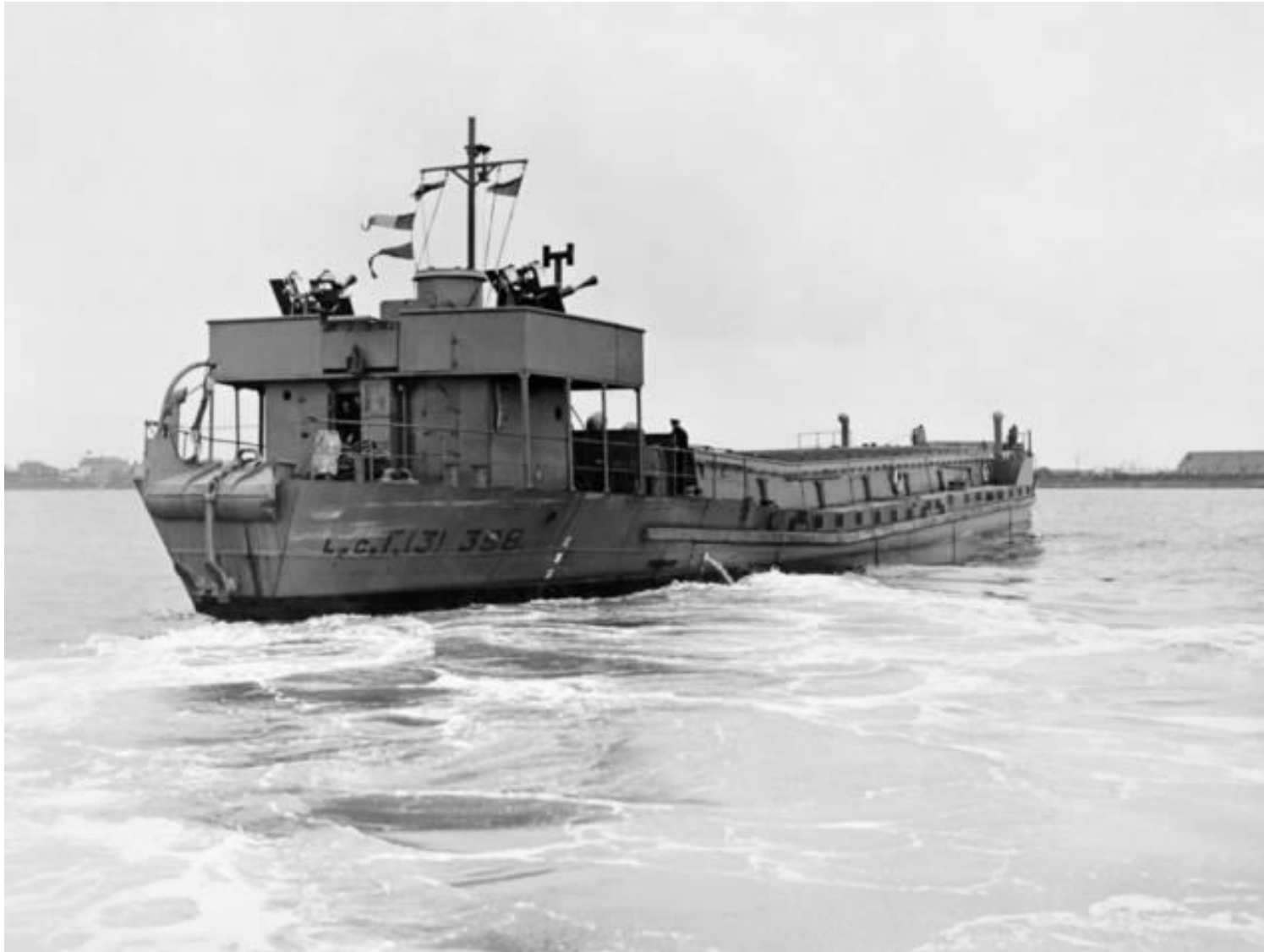
Figure 43 LCT Mk 3396 undergoing trials 1942. The guns are different than those found on LCT427. Image supplied under Licence from the Imperial War Museum.
