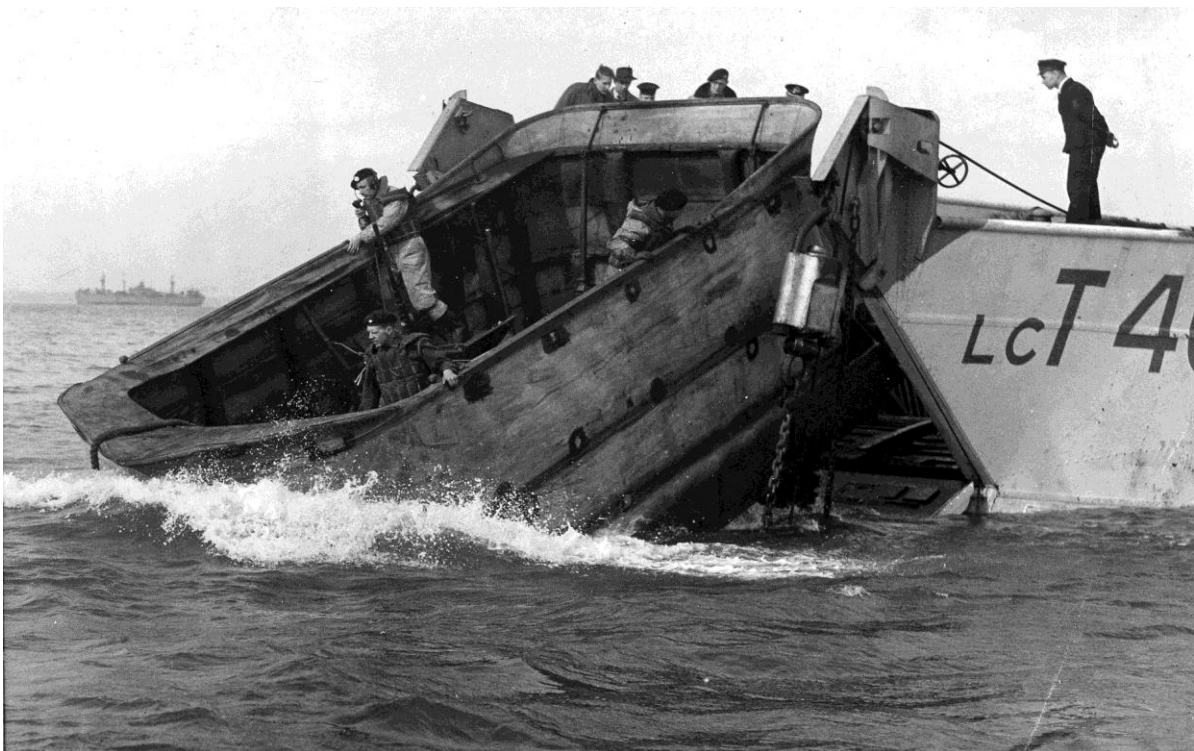
Figure 52 A Sherman DD tank being launched from a British LCT. Image courtesy of the Tank Museum Bovington.
